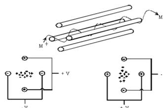
**Fig. 3: Quadrupole mass Analyzer**
