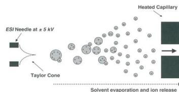
**Fig. 2: Schematic presentation of ESI process**
