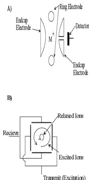
**Fig. 5: Ion cyclotron Mass Spectrometer**
