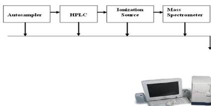
**Fig. 1: The components of an LC-MS system**
