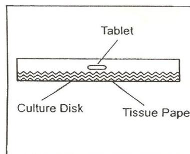
**Fig. 2: Schematic representation of wetting time /water absorption determination**
