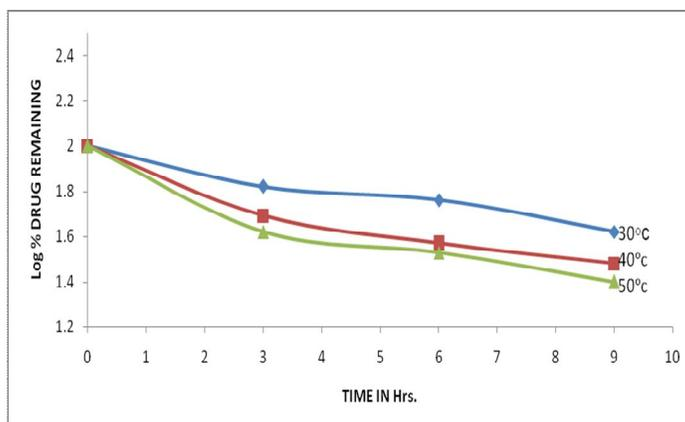
**Fig. 5 : First order plot of the oxidation of Phenobarbitone with 8% hydrogen peroxide at different temperature**
