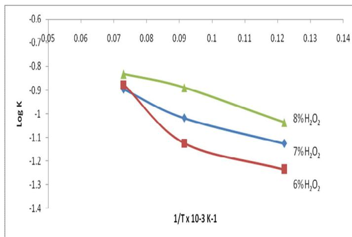
Fig. 7: Arrhenius plot for the oxidation of Phenobarbitone with 6%,7%,8% hydrogen peroxide
