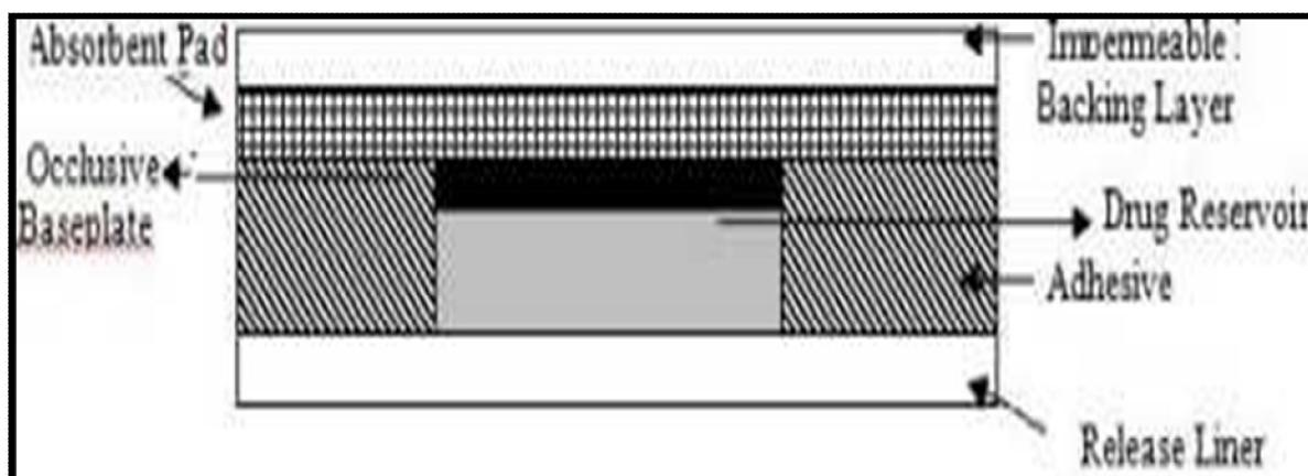
Fig. 4: Matrix-based transdermal patch
