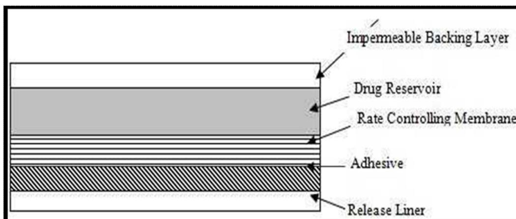
Fig. 3: Reservoir-based transdermal patch
