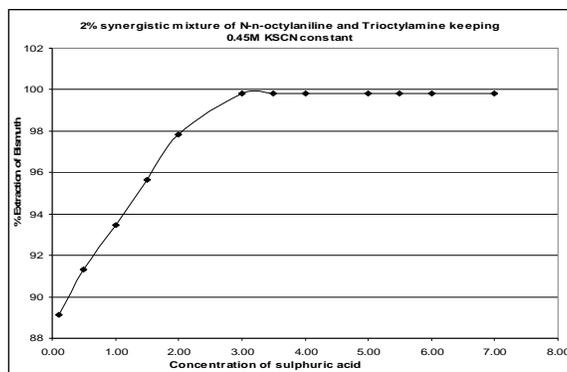
**Fig. 3:** Extraction behavior of Bismuth (III) with synergistic mixture of N-n-octylaniline and Trioctylamine concentration at 0.1 to 7.0 sulphuric acid and 0.4M potassium thiocyanate concentration.
