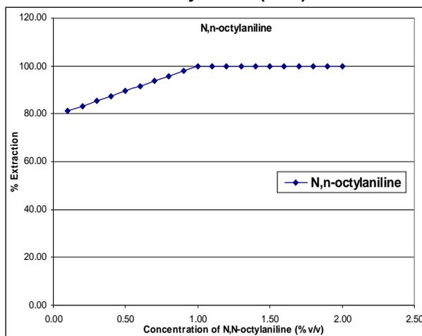
**Fig. 4b:** Extraction behavior of Bismuth (III) at fixed concentration of Trioctylamine (TOA) (1.0%), by varying the concentration of N-n-octylaniline.
