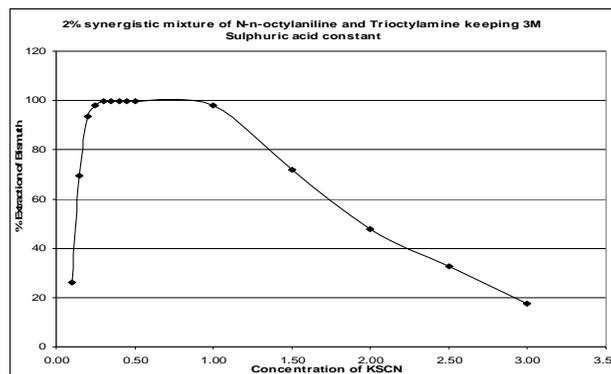
Fig. 2: Extraction behavior of Bismuth (III) with 2% synergistic mixture of N-n-octylaniline and Trioctylamine concentration at 0.1 to 3.0M potassium thiocyanate and 3M sulphuric acid concentration.
