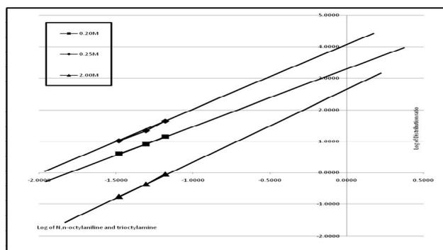
Fig. 1: Distribution Ratio of Bismuth (III) as function of synergistic mixture of N-n-octylaniline and Trioctylamine concentration at 0.2M, 0.25 and 2.0M potassium thiocyanate concentration
