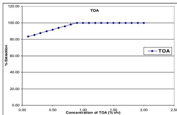
**Fig. 4a:** Extraction behavior of Bismuth (III) at fixed concentration of N,n-octylaniline (1.0%), by varying the concentration of Trioctylamine (TOA).
