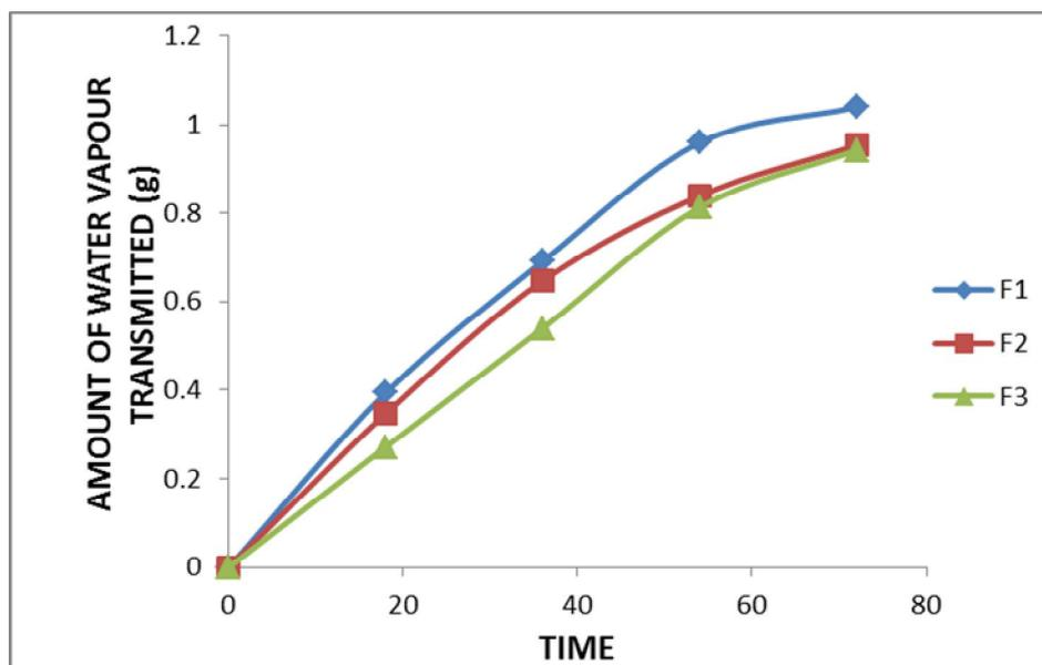
**Fig. 1: Water vapour transmission profiles of eudragit rlpo films casted with various solvents**
