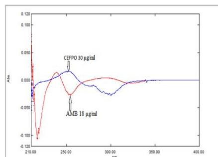
Fig. 2: Overlain first-order derivative spectra of AMB and CEFPO in 0.1 N HCl
