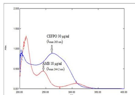
Fig. 1: Overlain zero-order absorption spectra of AMB and CEFPO in 0.1NHCl
