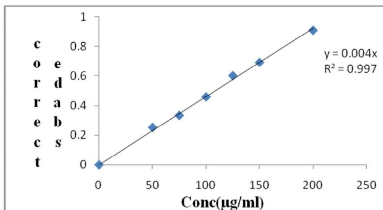
**Fig. 7: Rinse Recovery from SS Plate spiked with sample: Drug Conc./spiked part Vs Rinse Sample absorbance**
