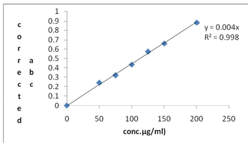
Fig. 5: Plate Recovery Study from Swabs Spiked on SS Plates: Conc. Vs corrected absorbance graph
