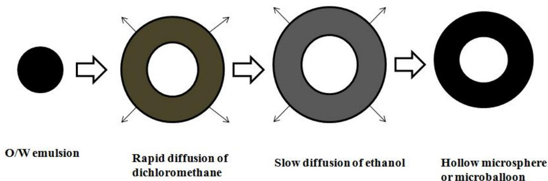
Fig. 5: Formulation of floating hollow microsphere or microballoon
