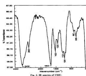
Fig. 2. IR spectra of CMC.
