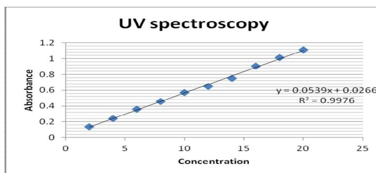
Fig. F: Zero order calibration curve of Didanosine
