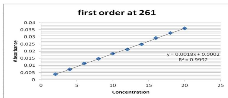
Fig. G: 1<sup>st</sup> order calibration curve of Didanosine
