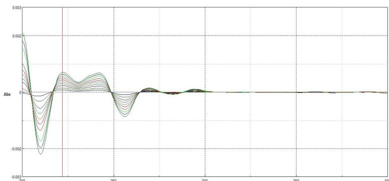
**Fig. D: Overlay spectra of third order derivative spectroscopy**
