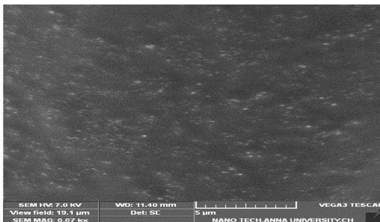
**Fig. 4: SEM of Iron particles at 5 microns**
