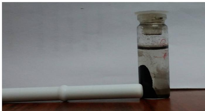
**Fig. 6: Biosynthesized Iron nanoparticles**
