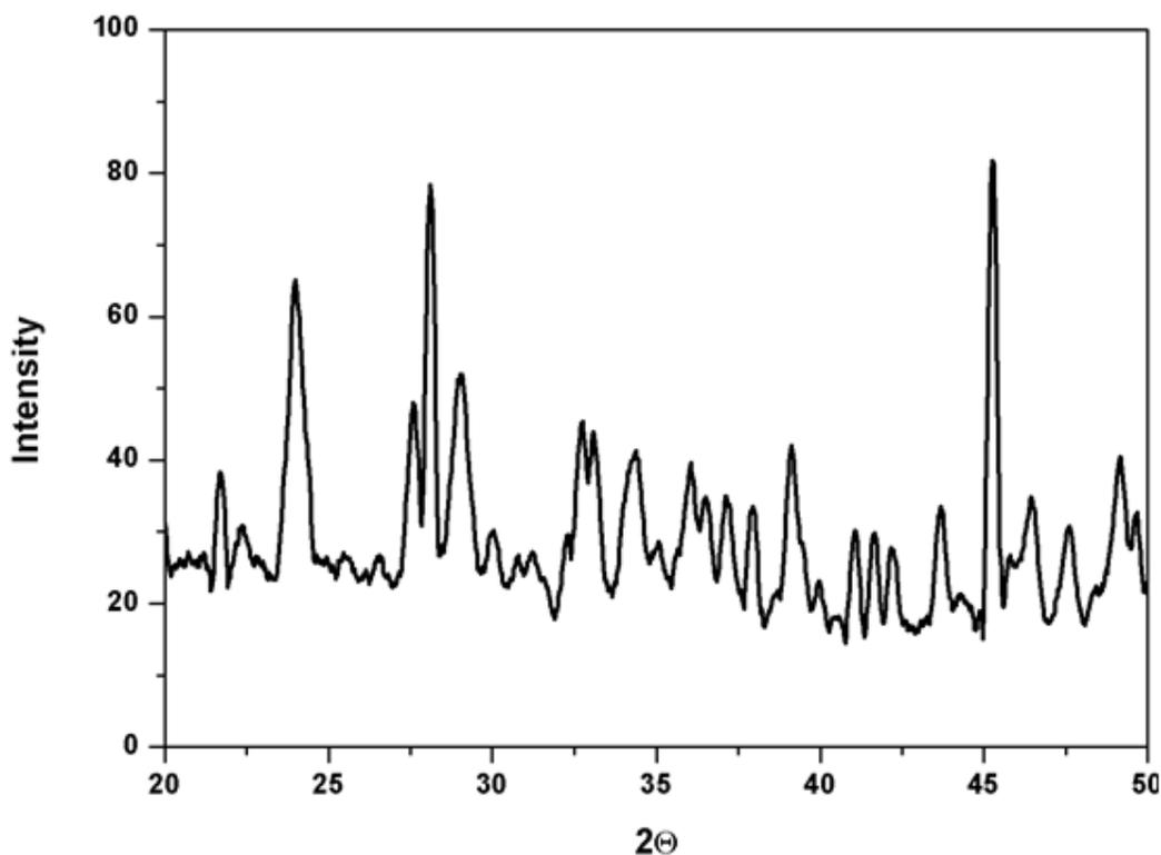
Fig. 3: XRD Pattern of Iron nanoparticles
