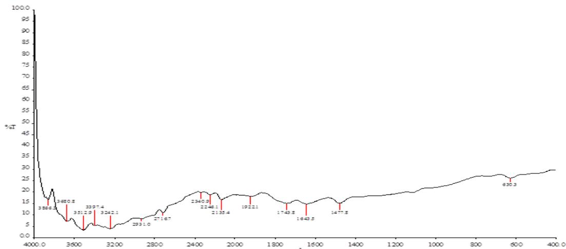
Fig. 2: FTIR analysis of Iron nanoparticles
