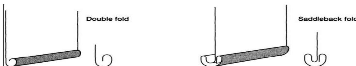
Fig. 3: Metal tube-end closures: typical folds<sup>1</sup>
