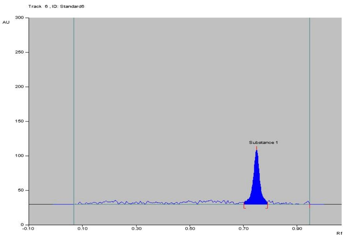
**Fig. 2: Densitogram obtained from sample solution of Eletriptan (600 ng/band;  $R_f = 0.76 \pm 0.01$ )**
