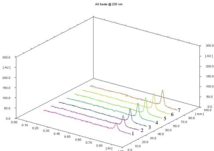
**Fig. 3: Three dimensional Chromatogram of Eletriptan (Peaks 1-6,(200-700ng/spot) of Standard eletriptan & Peak-7 of Sample)**
