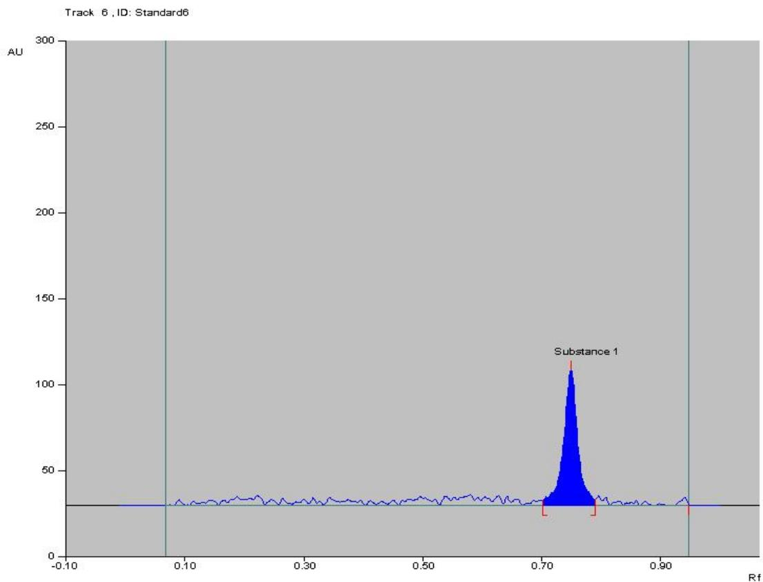
**Fig. 1: Densitogram obtained from a standard solution of Eletriptan (600 ng/band;  $R_f = 0.76 \pm 0.01$ )**
