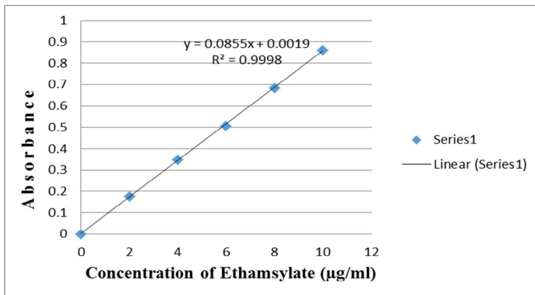
Fig. 3: Calibration Curve of Ethamsylate at 509nm
