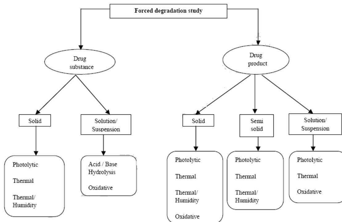
**Fig. 1: Flowchart describing various stress conditions for the degradation of the drug substance and drug product**
