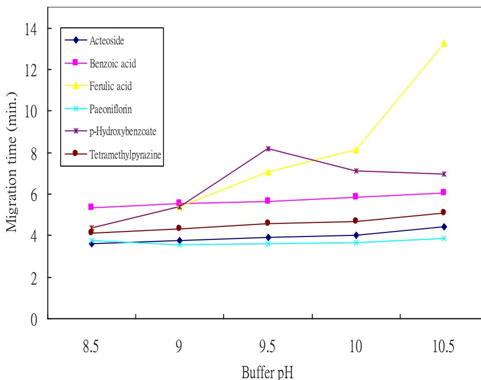
**Fig. 3: The effects of pH on migration times of marker components. ◆ Acteoside; × Paeoniflorin; ▲ Ferulic acid; ● Tetramethylpyrazine; ■ Benzoic acid; \* p-Hydroxybenzoate (internal standard).**
