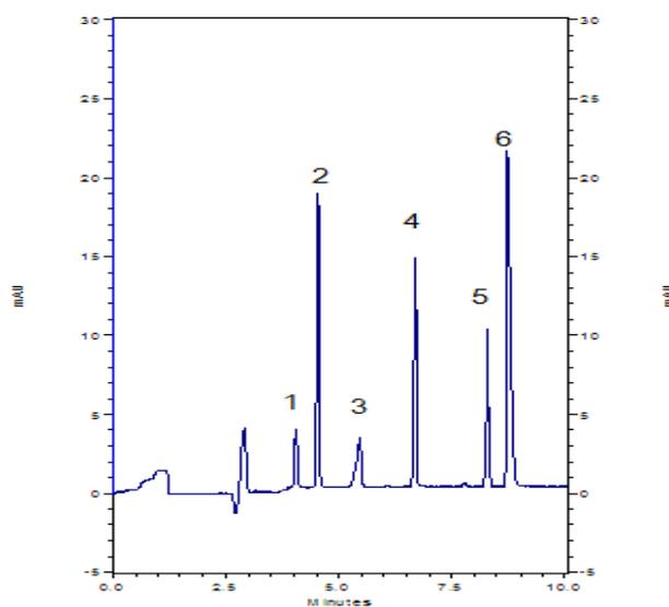
**Fig. 5 Electropherogram of five marker components in SWT. (1) Paeoniflorin, (2) Acteoside, (3) Tetramethylpyrazine, (4) Benzoic acid, (5) p-Hydroxybenzoate (internal standard) and (6) Ferulic acid. Electrophoresis conditions: 30 mM boric acid; 75 mM SDS; pH 10; fused silica capillary (50  $\mu$ m i.d.  $\times$  40 cm); applied voltage, 20 kV; run time, 10min; UV detection at 230 nm; temperature, 25  $^{\circ}$ C.**
