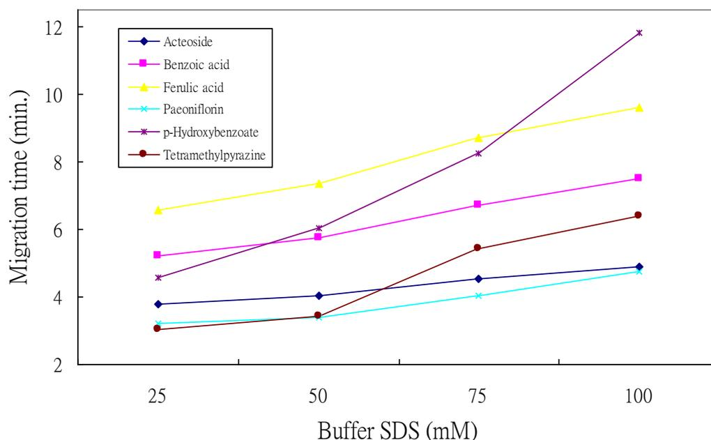
**Fig. 4: The effects of SDS concentration on migration times of marker components. ◆ Acteoside; × Paeoniflorin; ▲ Ferulic acid; ● Tetramethylpyrazine; ■ Benzoic acid; \* p-Hydroxybenzoate (internal standard)**
