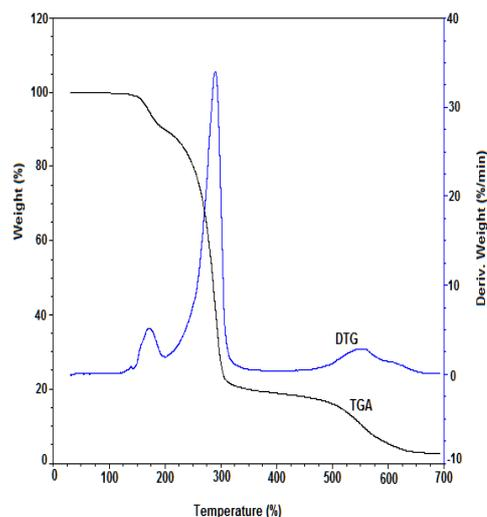
Fig. 2: Thermo gravimetric (TGA and DTG) curves of complex 2
