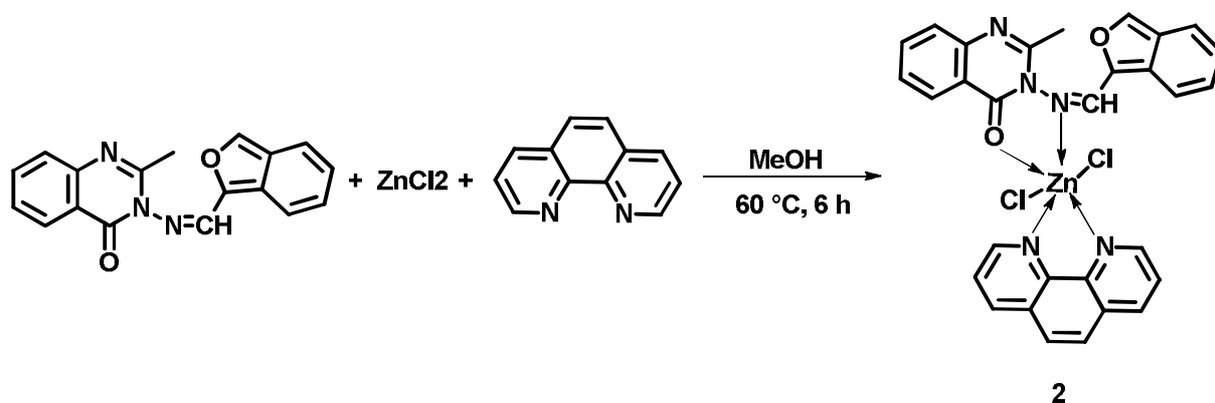
Fig. 1: synthetic route of 3-(isobenzofuran-1-ylmethyleneamino)-2-methylquinazolin-4(3H)-one (L) and its Zinc(II) complexes
