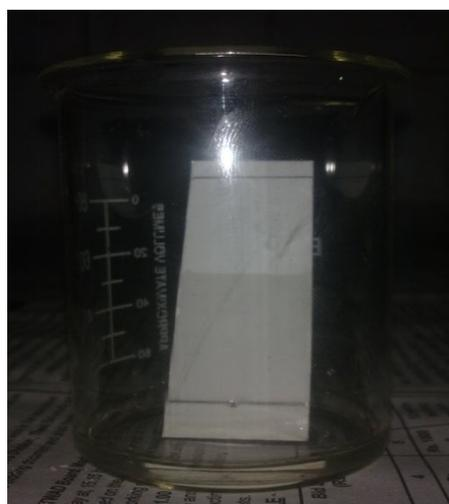
**Fig. 3: Thin layer chromatography development chamber**
