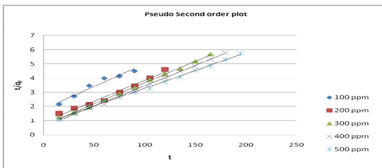
Fig. 11: The Pseudo Second order sorption kinetics for various initial concentrations
