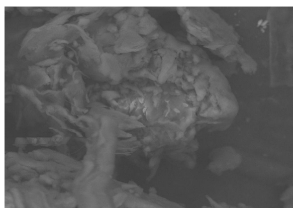
Fig. 3: SEM photograph of banana peel mucilage powder (2.0 k, Magnification)
