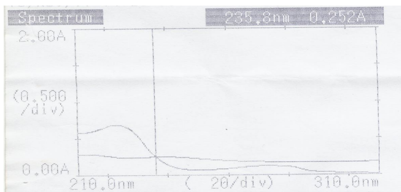
Fig. 1: Overlain spectra of synthetic mixture of Metoprolol and Amlodipine besylate between 210-310 nm
