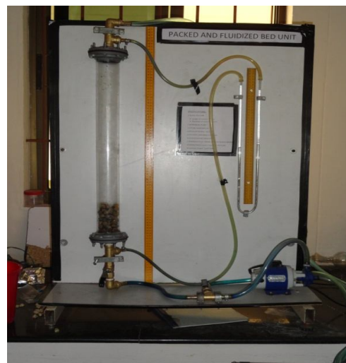
Fig. 1: Packed Bed Column with Maize Cob as Packing Material
