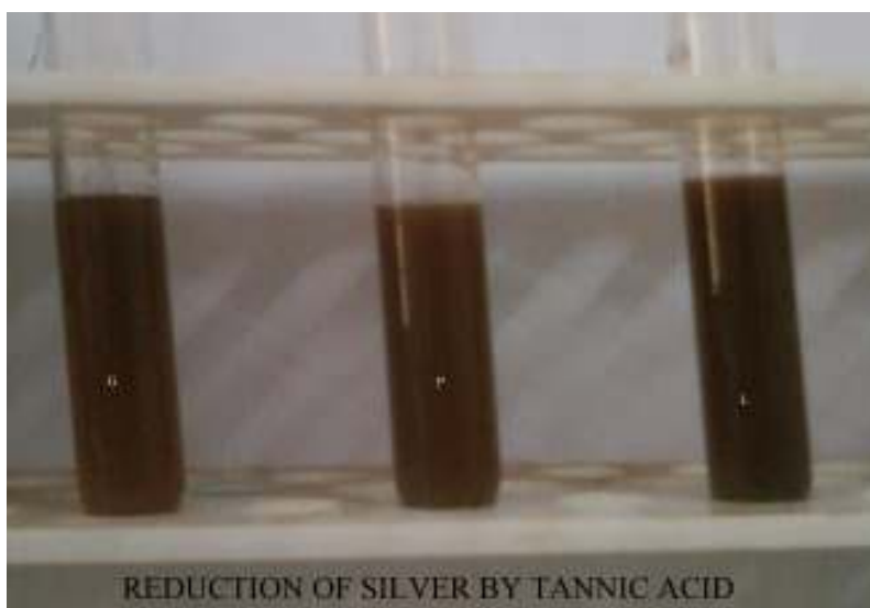
Fig. 8: The reduction of silver nitrate to silver nanoparticles using purified compound of tannic acid
