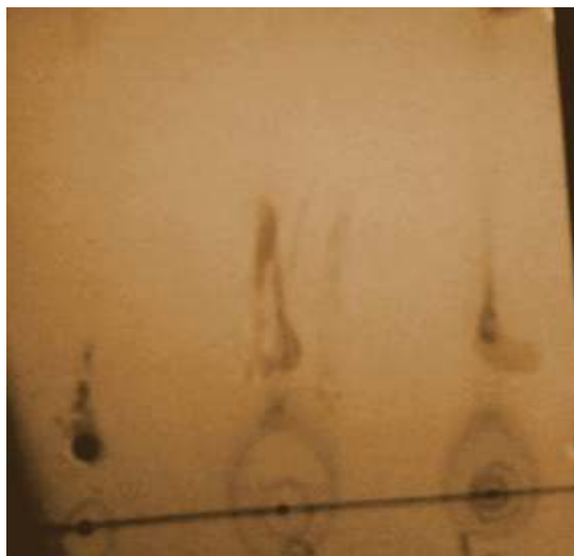
Fig. 4: TLC plate showing the presence of flavonoids
