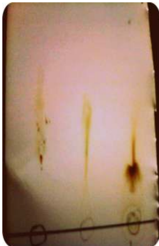
Fig. 7: TLC plate showing the confirmation of tannin
