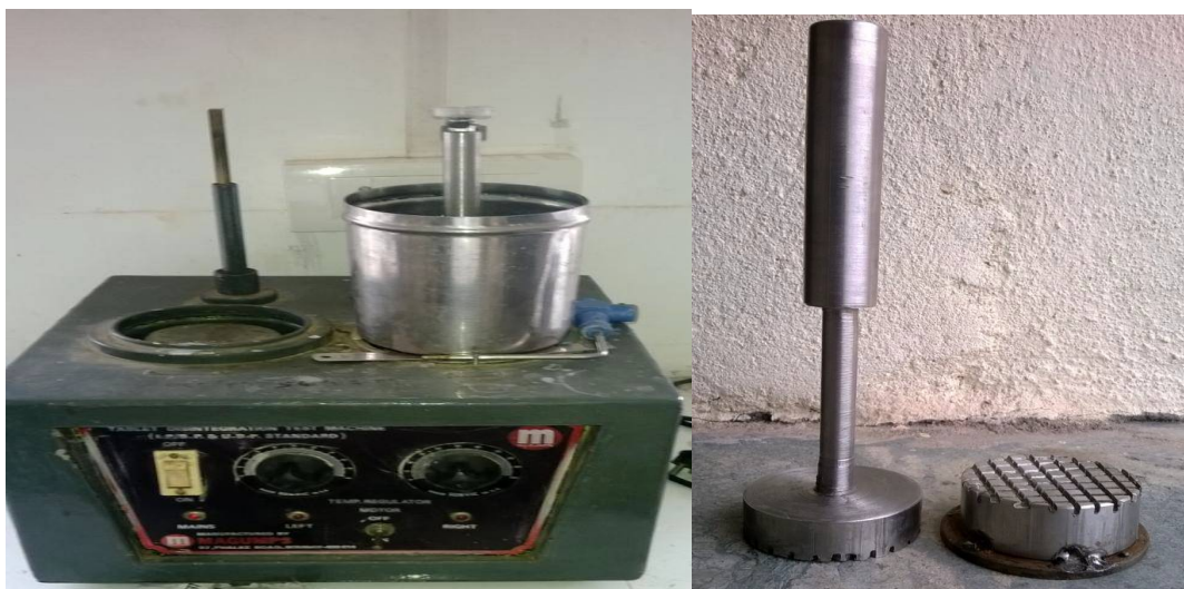
Figure 2: Lab fabricated herbal chewing gum apparatus with S.S die and punch. Release measurements were performed using lab fabricated herbal chewing gum test apparatus at 50 rpm. In each flask a 900ml of artificial saliva pH 6.4 was filled. The temperature was maintained at 37 °C. At predetermined interval (0, 2, 4, 6, 8, 10, 12 and 14)(min) absorbance was recorded spectrophotometrically at 280nm and the percentage of drug released was determined as a function of time
